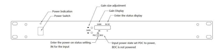
Gain Button: You can adjust the gain size, you can adjust the controller gain increase or decrease. Digital Display: The display can be on the gain value, input status display.
